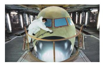
Dustcontrol was entrusted with supplying four stationary systems with on-tool extraction.
